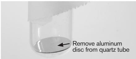
To remove the aluminum disc in older Ultra UV units do one of the following.
